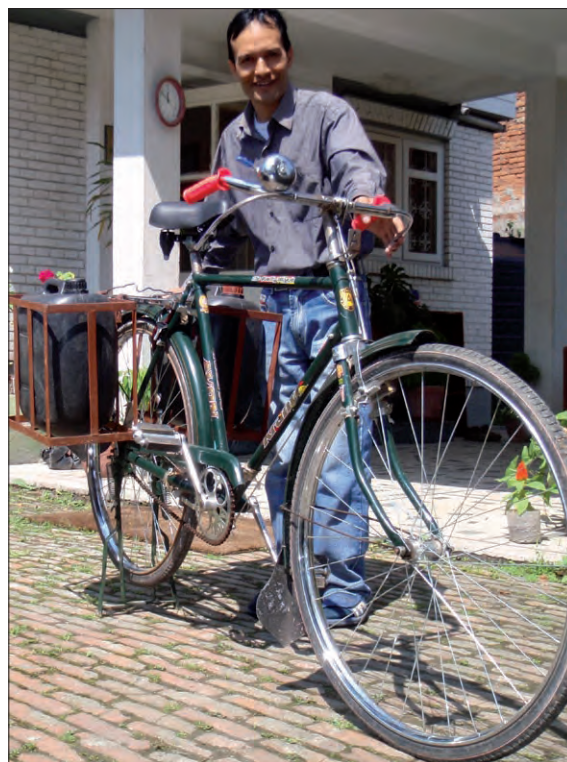
The 'pee-cycle' used for urine collection from about a dozen households in Siddhipur
